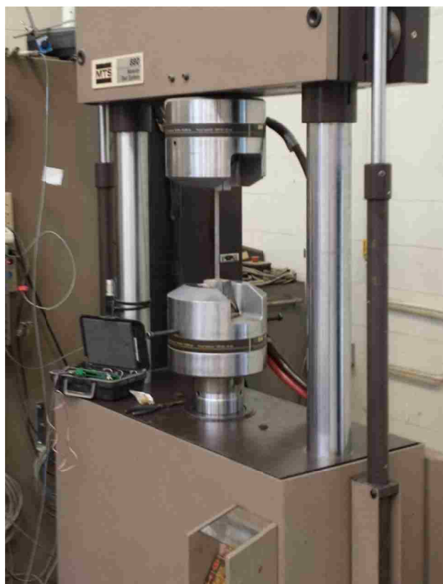
Figure 3.1 Typical Tensile Coupon Test Setup
