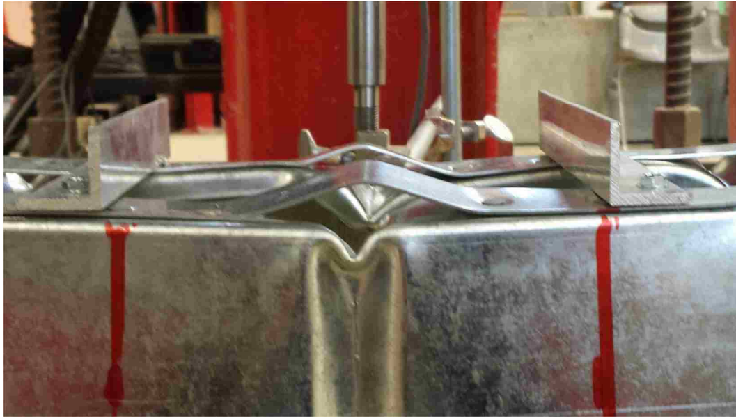
Figure 4.4 Typical Failure of Crimp in Compression with Reinforcing Band
